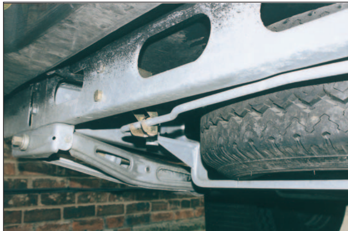
The spare wheel cradle has been relocated for easier retrieval; corner steadies are standard.
