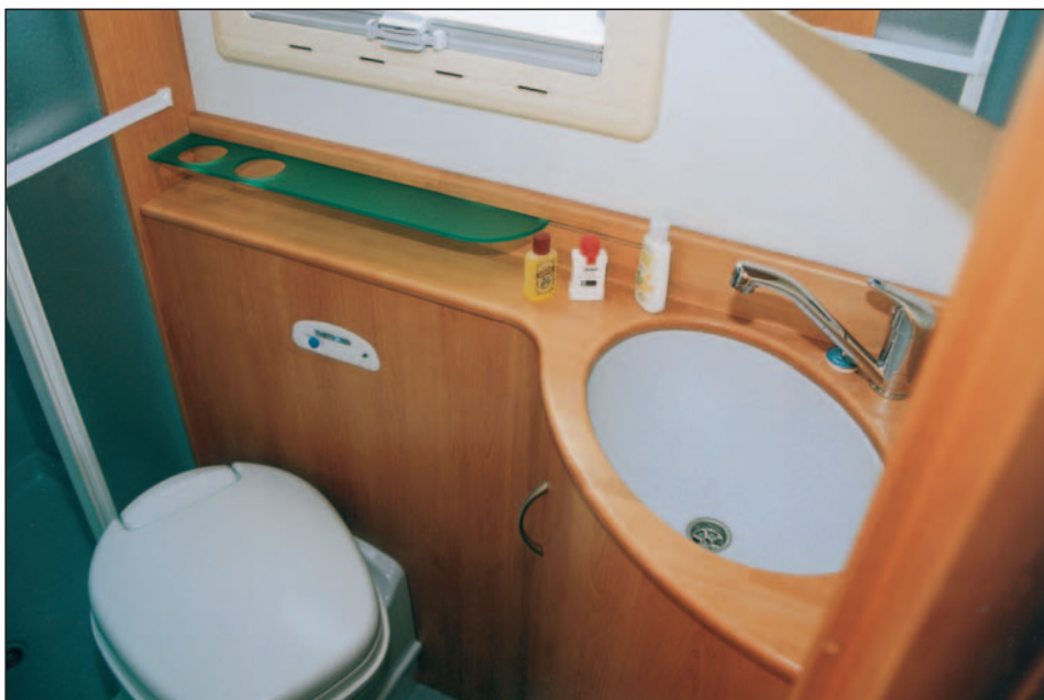
Well-equipped washroom has an electric-flush swivel-bowl loo and a vanity sink inset into a smart wooden cabinet.
